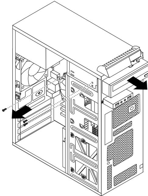
Figure 18. Removing the optical drive
