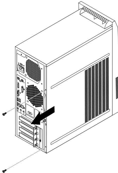
Figure 9. Removing the computer cover
