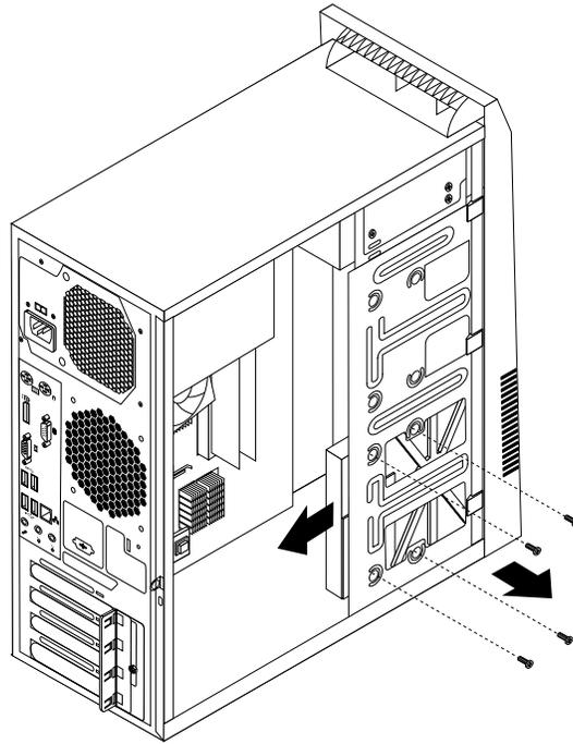
Figure 29. Removing the hard disk drive
