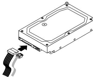
Figure 31. Connecting a SATA hard disk drive
