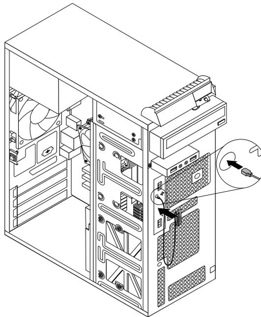
Figure 46. Installing the front WiFi antenna
