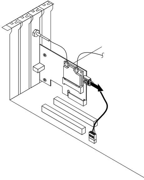
*Figure 35. Disconnecting the Bluetooth cable*
