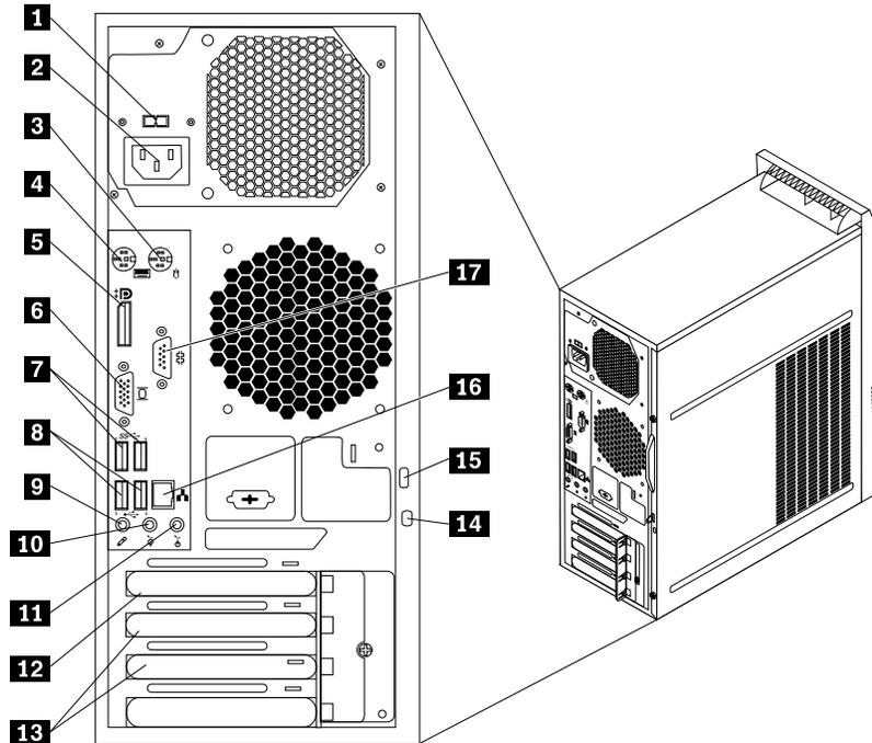
Figure 2. Rear connector locations
