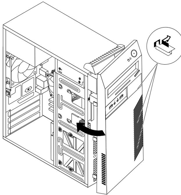
Figure 11. Reinstalling the front bezel
