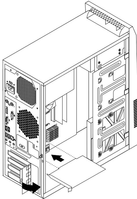
Figure 14. Installing a PCI Express card
