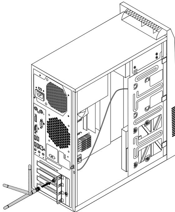
Figure 43. Installing the rear WiFi antenna
