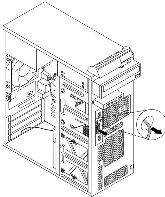
Figure 47. Removing the front WiFi antenna
