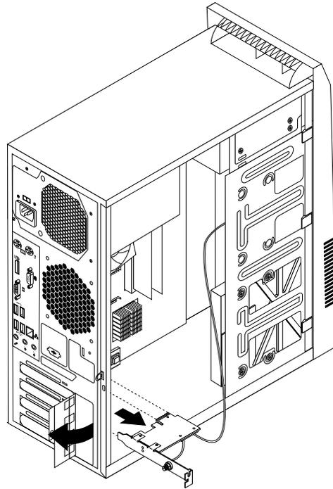
Figure 36. Removing the WiFi adapter card
