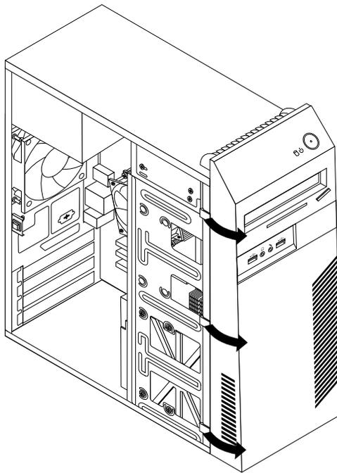
*Figure 10. Removing the front bezel*
