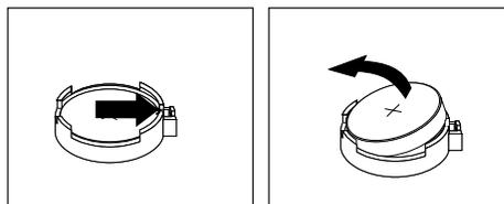
Figure 21. Removing the old battery
