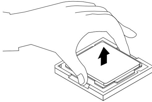
*Figure 26. Removing the microprocessor*
