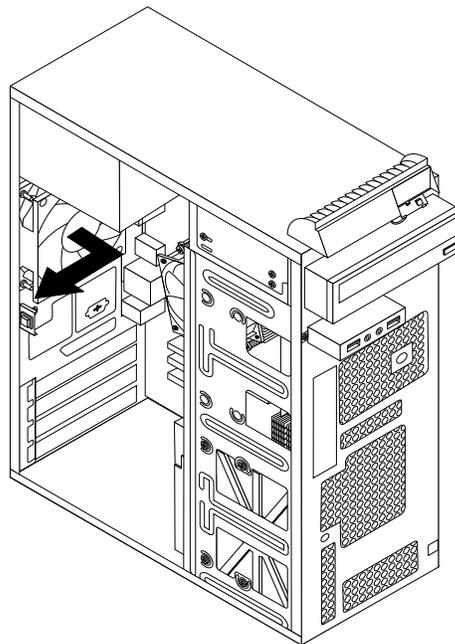
*Figure 32. Removing the rear fan assembly*
