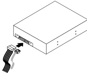
Figure 20. Connecting a SATA optical drive
