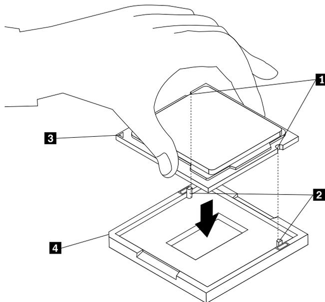
Figure 27. Installing the microprocessor
