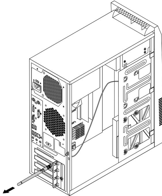
Figure 44. Removing the rear WiFi antenna
