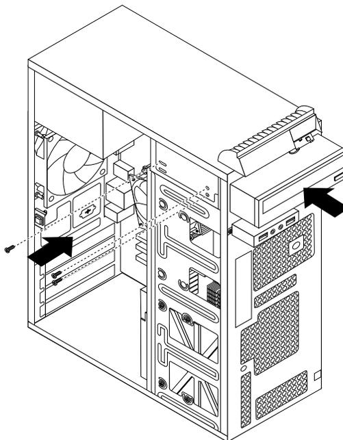
Figure 19. Installing the optical drive
