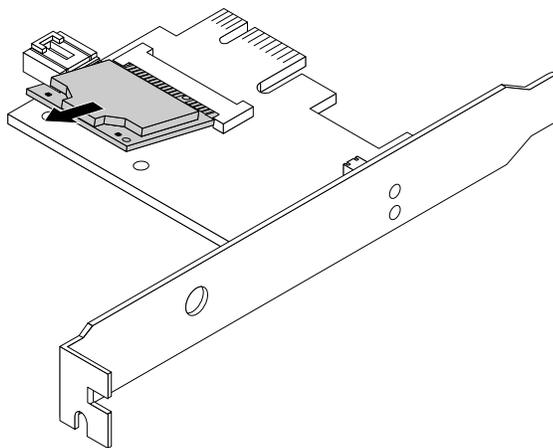
*Figure 39. Removing the WiFi card module*
