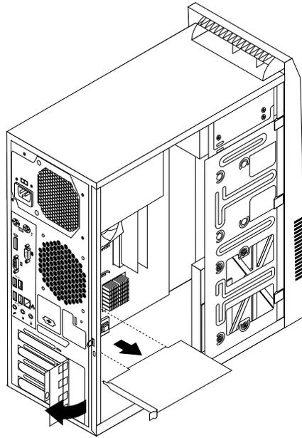
Figure 13. Removing the PCI Express card
