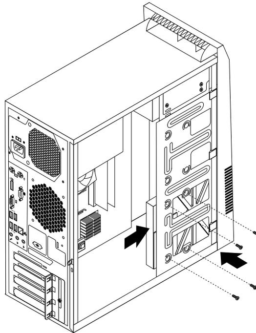
Figure 30. Installing the hard disk drive
