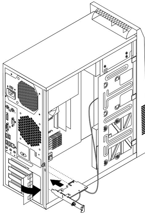
Figure 42. Installing the WiFi adapter card
