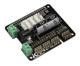
The MotoPi board is an expansion board for controlling and using up to 16 PWM-controlled 5V servo motors. Its own clock on the MotoPI provides a very accurate PWM signal and also a precise positioning. The built-in capacitor additionally buffers the current. This reduces the collapse of the stress in the event of a brief additional load, which could otherwise lead to jerking. An additional capacitor can also be connected.
